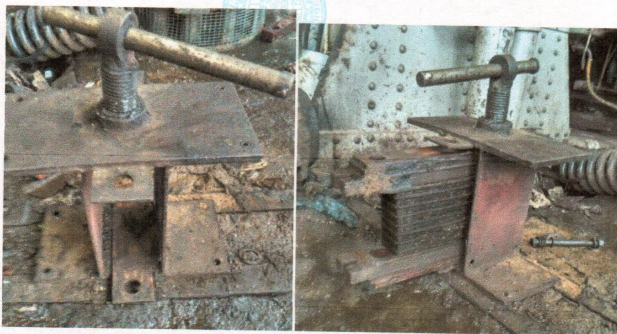
Fig.2: fixture for pressing SMU for fitment in locomotive
